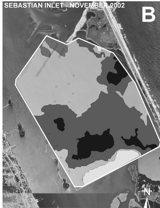
Fig. 3. Survey results near Sebastian Inlet on 50 kHz. Black=dense algae, medium grey=sparse algae, light grey=bare seafloor, striped=seagrass. Groundtruthing locations for the calculation of confusion matrices in Table 1 are indicated as black circles.
